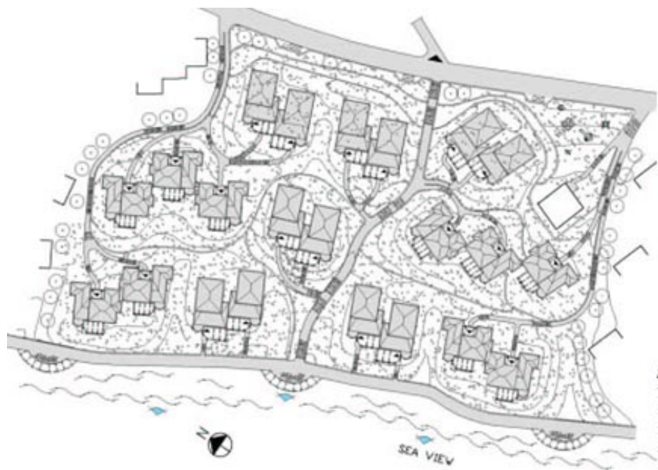
Site Plan The position of each house was taken on the site in relation to the others, so to ensure an open view to the sea.
