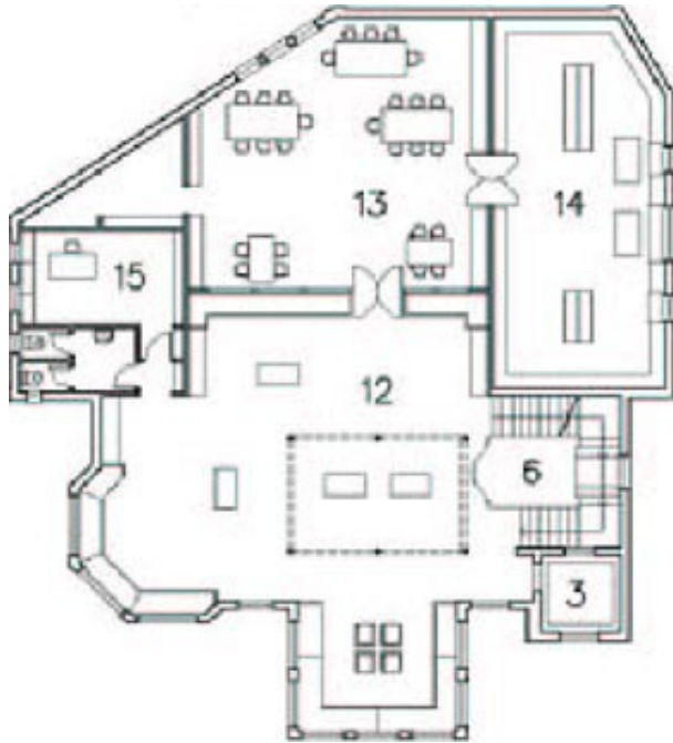
second floor plan 12 museum of music 13 study and periodicals room 14 archive 15 curator's room
